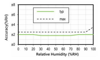
${\it 3. \ Typical \ RH \ accuracy \ corresponding \ to \ the \ temperature:}\\$
