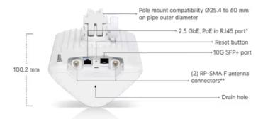
\*48V DC, 0.65A 2.5 GbE PoE adapter included. \*\*For external 5 GHz antenna (optional).
