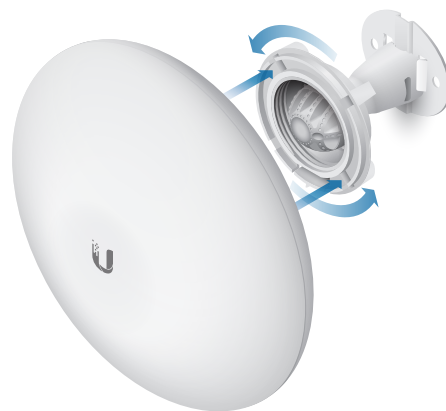
Installation Using the NanoBeamM Wall Mount Kit
