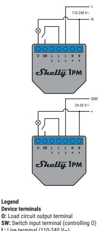
0: Load circuit output terminal SW: Switch input terminal (controlling 0) L: Live terminal (110-240 V~) N: Neutral terminal +: 24-30 V--- positive terminal L: 24-30 V--- negative terminal Wires L: Live wire (110-240 V~) N: Neutral wire +: 24-30 V- positive wire GND: 24-30 V--- ground wire
