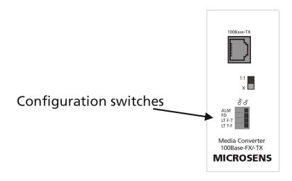
To ensure that the network management can read the connection status, the converter has additional integrated features such as Link Through and Advanced Link Monitor (ALM). The Link Through forwards the connection status to the converted segment. Due to this the fiber port is interrupted if the twisted pair connection fails and vice versa.
