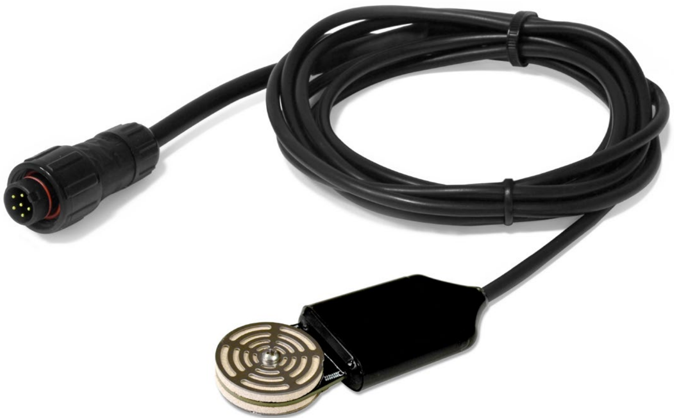
Figure: Soil water potential sensor probe (Decagon MPS-6)
