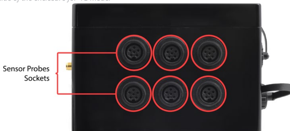
Figure: Sensor side of the enclosure
