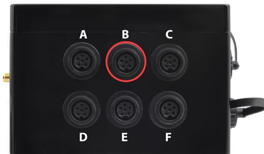
Figure: Available sockets for the Phytos 31 sensor probe
