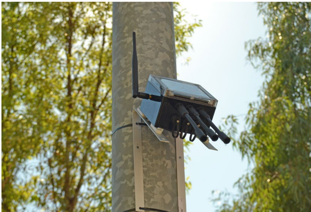
Figure: Waspote Plug & Sense! powered by an internal solar panel
