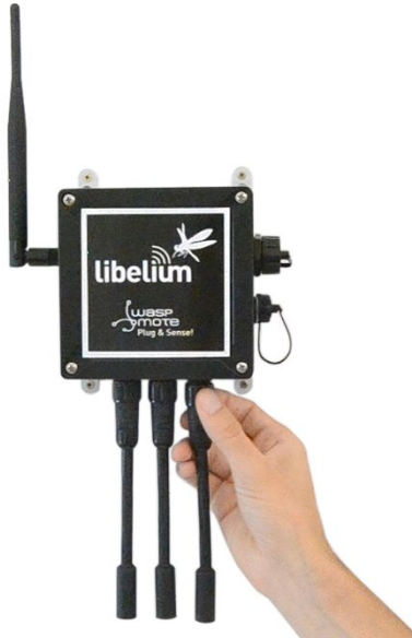
Figure: Connecting a sensor probe to Waspote Plug & Sense!
