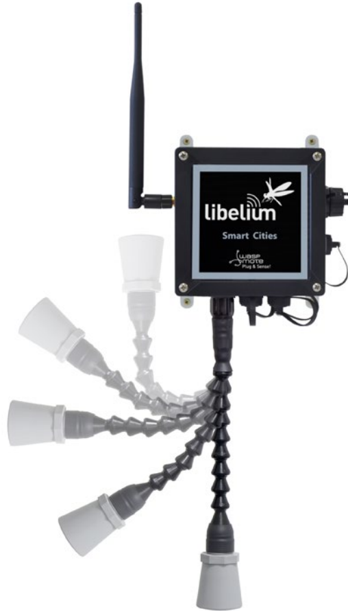
Figure: ultrasound sensor (Maxbotix MB7040) installation
