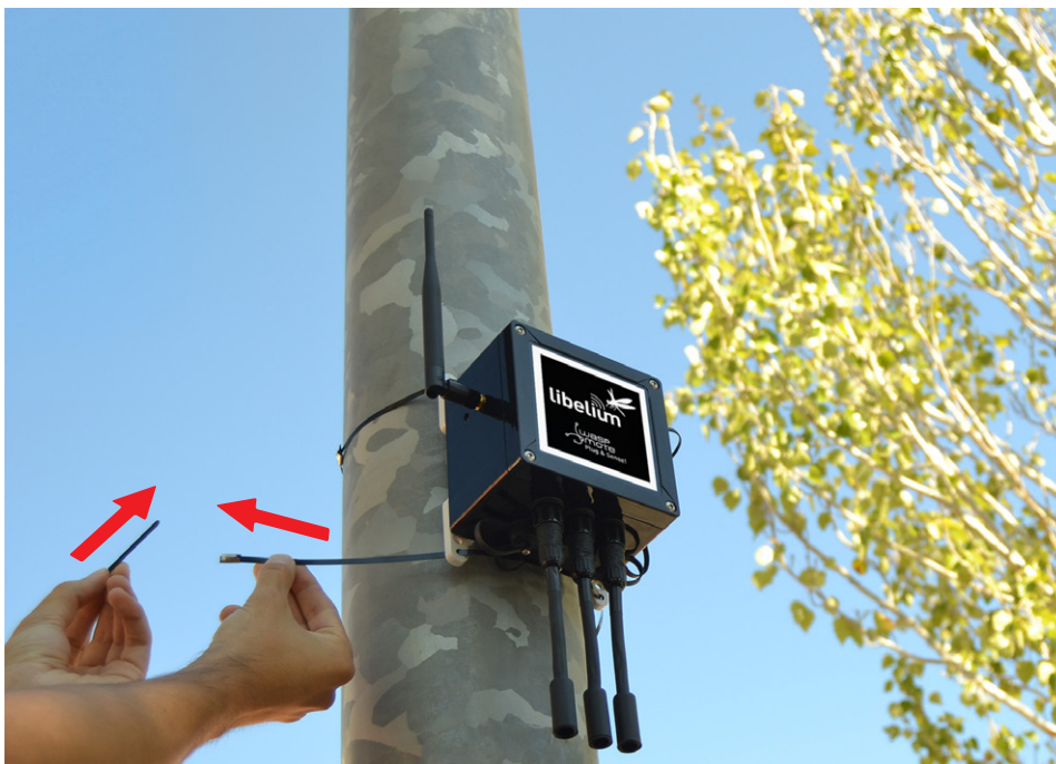
Figure: Placing Waspote Plug & Sense! on a street light
