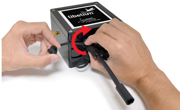
Figure: Connecting a sensor probe to the enclosure
