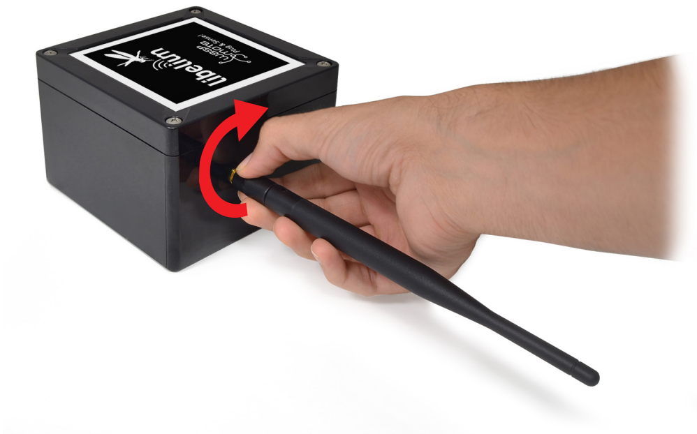
Figure: Connecting antenna to the enclosure
