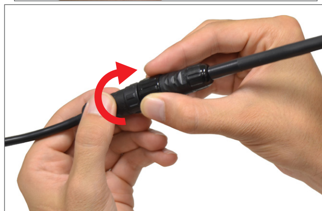
Figure: Connecting a probe with an extension cord
