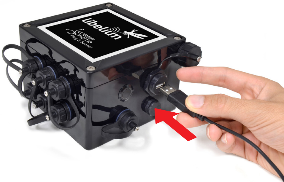
Figure: Connecting the USB cable to Wasp mote Plug & Sense!
