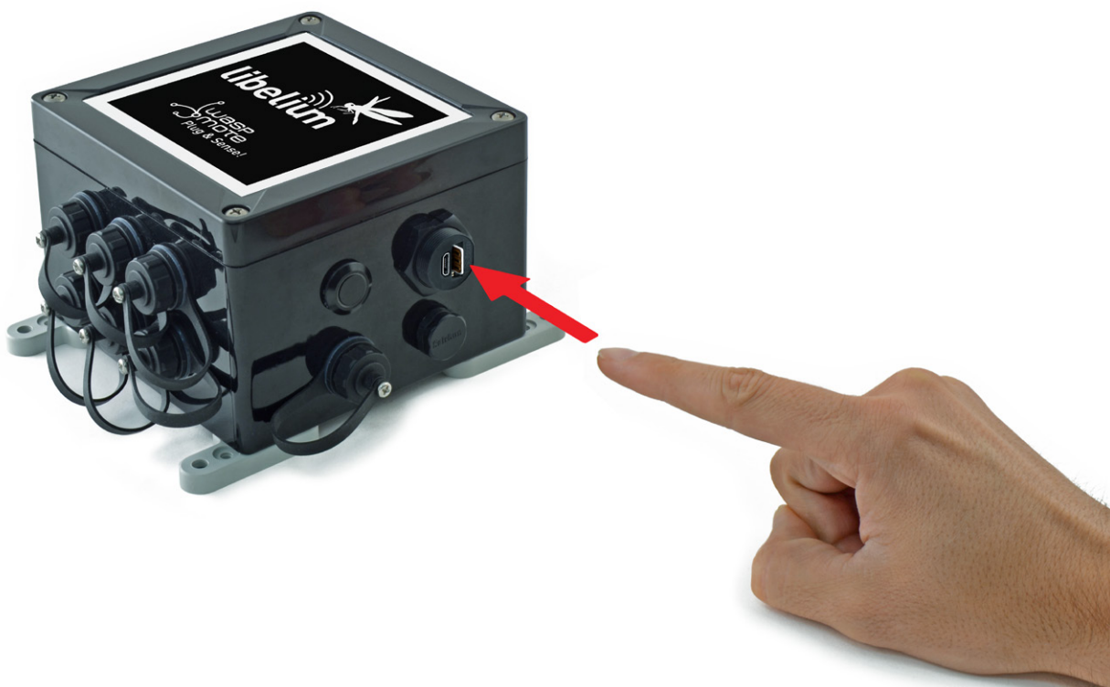
Figure: Inserting a SIM card with care in the External SIM/USB socket
