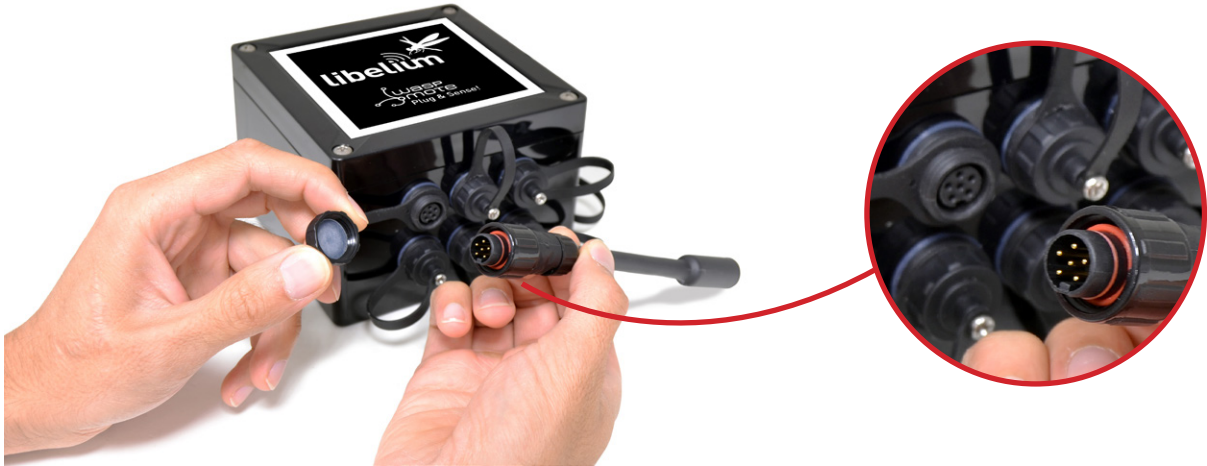
Figure: Detail of sensor waterproof connector
