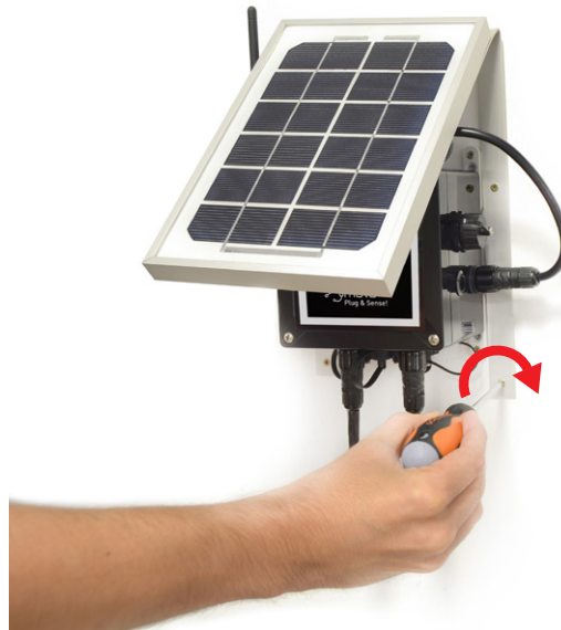
Figure: Placing the external solar panel above Wasp mote
