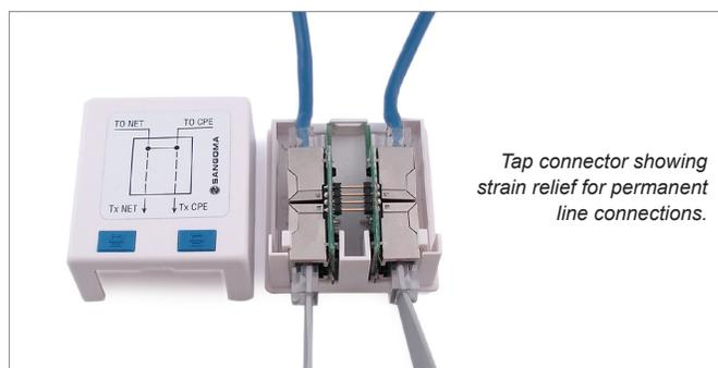
The system can be used in both standard impedance and high impedance modes, high impedance being used to ensure that no accidental short of the monitoring lines will affect the flow of T1/E1 traffic.
