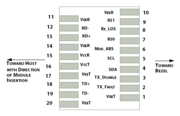
Figure 1: Interface to Host PCB
