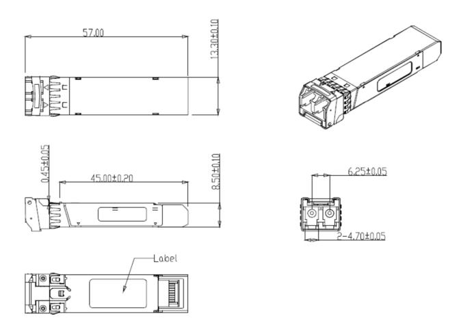
Figure 5. Mechanical Specifications
