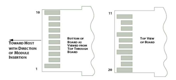
**Figure 2: Module Contact Assignment**
