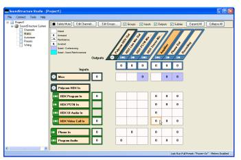
The matrix page (above) shows the signal routing from inputs to outputs for all audio channels in the system. Groups of multiple signals can be collapsed and configured as a single channel or expanded and configured individually.
